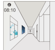
When the natural light level exceeds off set-point, the light will turn off even if when the space is occupied.
