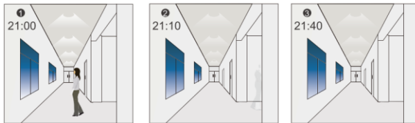
The light switches on at 100% when there is movement detected.
